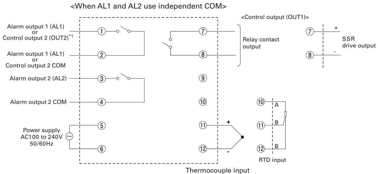
\*1: During dual control, the alarm output 1 functions as the control output 2.
