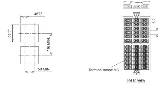
Terminal block is not attached to unused terminals (terminal 13 to 24) according to the model.
