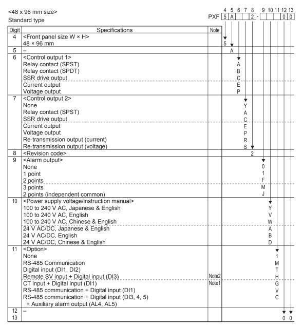
Note 1: When using the CT input as a heater burnout alarm, add one alarm output for it in the 9th code. Note 2: When using the current input for the remote SV input, add a 250-ohm resistor to the input terminal.
