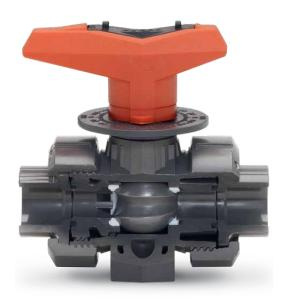
The Type 523 Metering Ball features a V-notch design. This type of ball design allows for flow control even at very low flow rates given the size of the valve. The flow characteristics curve is nearly linear because orifice size changes gradually as the valve is opened and closed. This type of V-notch design provides much better flow control, especially at low flow rates, when compared to both keyed orifices and 90° V-notch flow control balls.
