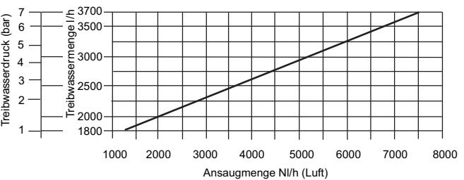
**DN40, nozzle size 3.5**
