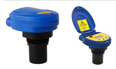
The general purpose ultrasonic level transmitter provides continuous level measurement up to 32.8' (10m) with a 4-20 mA signal output, and is configured via its integral push button display module. This noncontact liquid level sensor is ideally suited for corrosive, ultrapure, sticky or dirty liquids, and is broadly selected for bulk storage, day tank, lift station and process tank level applications.
