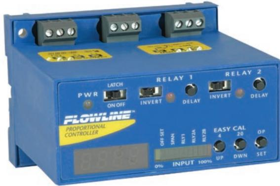
The general purpose controller provides single tank level indication with 2 relays, 1-3 set points and an isolated analog repeater. Relay 1 is configurable on a single set point. Relay 2 can be configured on a single set point or latched on two set points for automatic fill or empty control. Package the controller with any of our level transmitters. The NEMA 4X polycarbonate enclosure is a great choice for field mount installations and comes complete with a DIN rail mounting kit.
