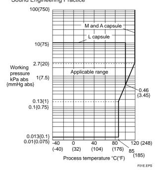
Figure 1. Working Pressure and Process Temperature
