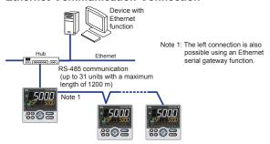
An Ethernet connection is also possible using controllers with an RS-485 communication function and an Ethernet/RS-485 converter (Yokogawa VJET is recommended).
