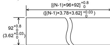
"N" stands for the number of controllers to be installed. However, the measured value applies if N≥5.
