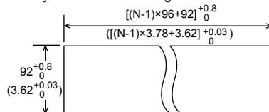
"N" stands for the number of controllers to be installed. However, the measured value applies if N ≥ 5. Normal tolerance: ±(value of JIS B 0401-1998 tolerance class IT18)/2
