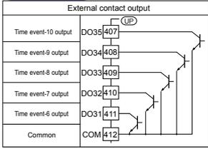
Transistor contact rating: 24 V DC, 50 mA
