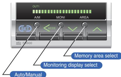
Pressing the MODE select key for 2 sec enables the same mode selection as in the conventional REX-F900/F400.
