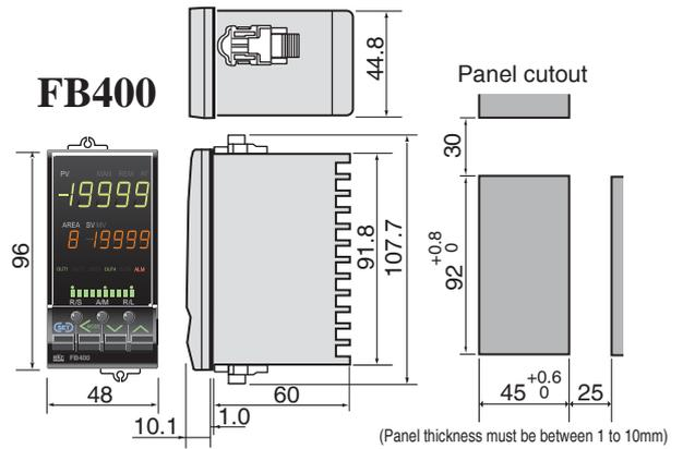
(Panel thickness must be between 1 to 10mm)
