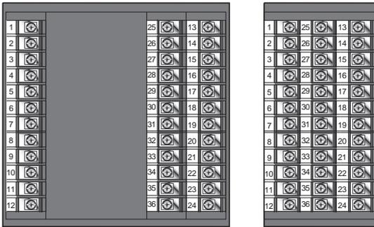
• Use a solderless terminal for screw size M3X6.
