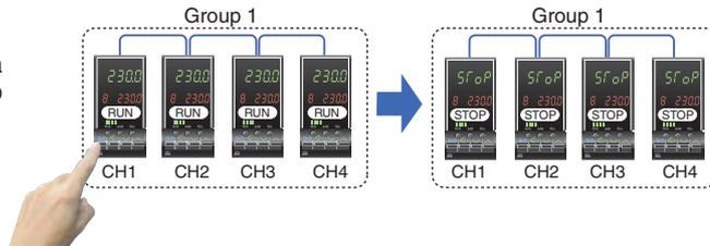
(Note) Time lag among controllers caused by inter-controller communication is (Max.70ms) x (number of controllers connected). Please consider the time lag of inter-controller communication for high-speed process control in which process changes rapidly.
